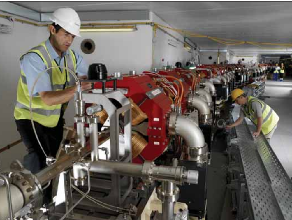
Fig 5 Once the stream of electrons enter the large 560 m diameter storage ring, they begin to give off synchrotron radiation
