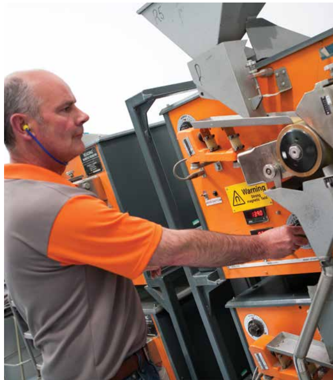
At the Element Six Micron+ Production Centre the incoming synthetic diamond is magnetically separated, milled to shape and size. The micron is then cleaned and rinsed before sedimentation.
