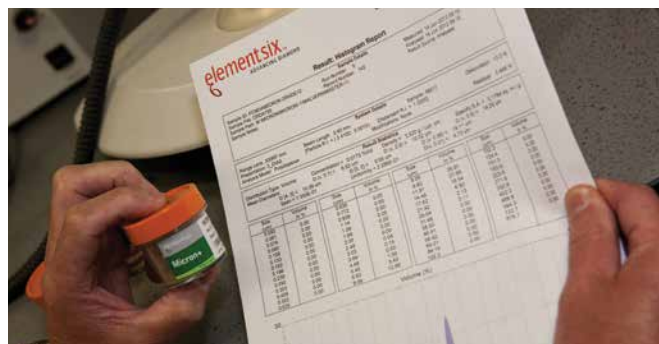
Throughout the manufacturing process, the Micron+ is monitored by visual inspection and laser diffraction to make sure every batch matches each individual customers' exacting specification requirements.
